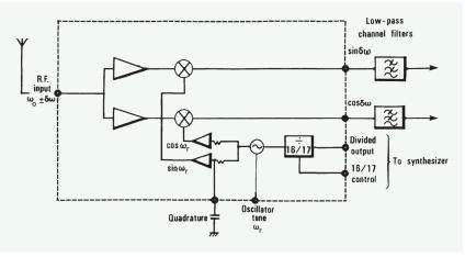
FIGURE 12: An integrated direct-conversion RX from 1980 [34].
