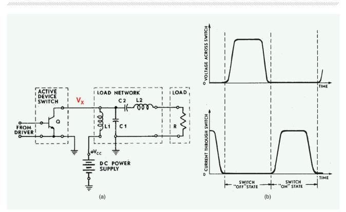
FIGURE 11: (a) The class-E stage proposed by Sokal and Sokal [21] and (b) its nonoverlapping current and voltage waveforms. (Red text added for illustration.)
