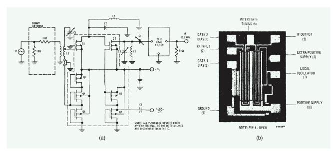
FIGURE 9: (a) A CMOS RX from 1969 [14] and (b) its die photograph.
