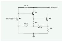
FIGURE 14: An integrated 1-GHz LNA from 1989 [36]
