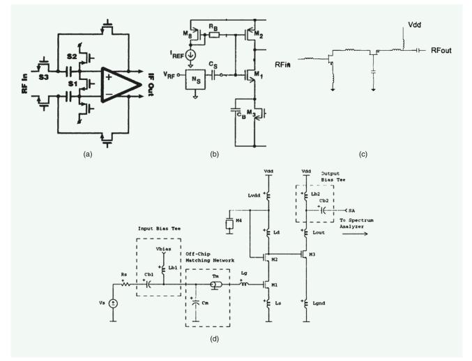
FIGURE 17: (a) A CMOS mixer from 1993 [43], (b) an inverter-based LNA from 1996 [44], (c) a MESFET LNA from 1993 [45], and (d) a CMOS LNA from 1996 [46]. (Parts of diagrams omitted for clarity.)
