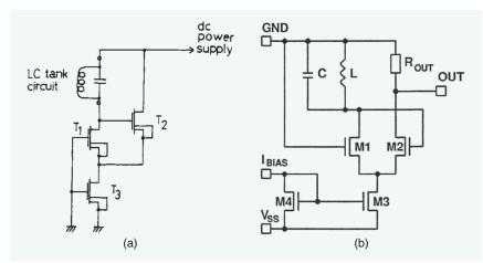
FIGURE 8: (a) A CMOS oscillator from 1968 [12] and (b) its counterpart from 1994 [13].
