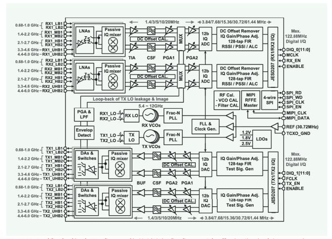
FIGURE 30: A multiband multimode LTE radio reported in 2018 [105]. Adj.: adjustment; Cal.: calibration; Sig.: signal; Gen.: generation; CLK: clock.
