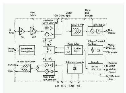
FIGURE 16: Siemens' 1994 direct-conversion transceiver [42].
