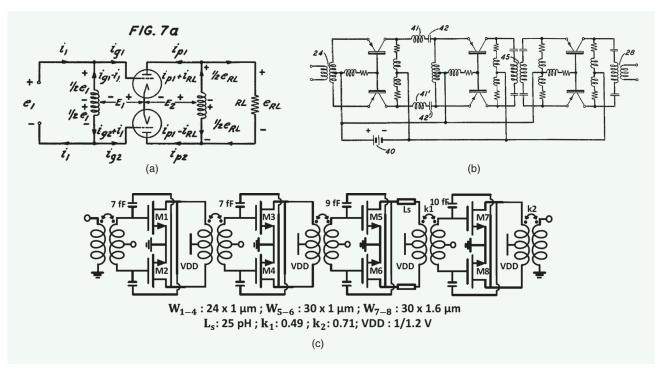
FIGURE 1: (a) A vacuum-tube amplifier [3], (b) its multistage transistor counterpart [3], and (c) a modern example [4].
