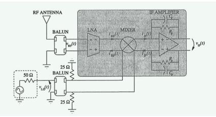
FIGURE 26: An RX chain consisting of a current-mode mixer and a TIA from 2003 [73].
