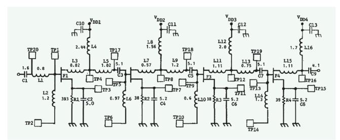
FIGURE 13: An LNA with interstage matching [35]. TP: test point.
