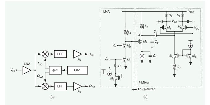
FIGURE 24: (a) A direct-conversion CMOS RX from 1997 [62] and (b) its front-end implementation.
