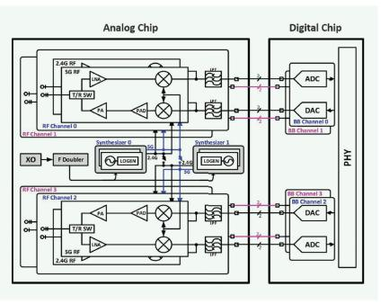
FIGURE 31: An IEEE 802.11ax radio reported in 2020 [106]. LPF: low-pass filter; PAD: PA driver; SW: switch.
