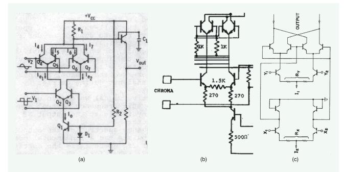
FIGURE 10: (a) A mixer reported by Bilotti and Pepper [18] in 1967, (b) an improved mixer reported by Bilotti [19] in 1968, and (c) a multiplier proposed by Gilbert [20] in 1968. (Parts of diagrams omitted for clarity.)
