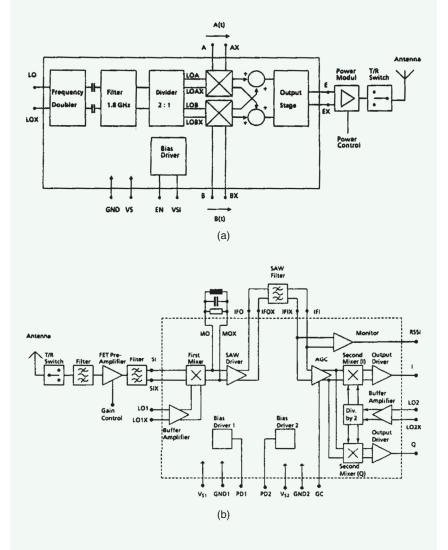
FIGURE 15: Siemens's 1990 (a) TX and (b) RX paths [41]. Div.: divider.
