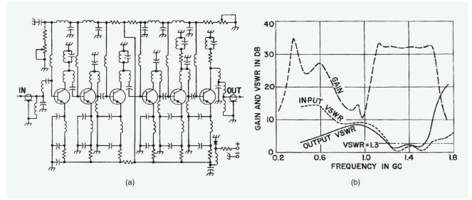
FIGURE 4: (a) A gigahertz amplifier from 1963 [7] and (b) its frequency response. GC: gigacycles per second (GHz).
