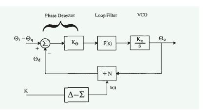
FIGURE 23: The  $\Delta\Sigma$  modulator proposed by Riley et al. [53].
