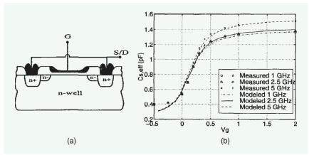
FIGURE 19: (a) The MOS varactor structure and (b) its characteristics [48].
