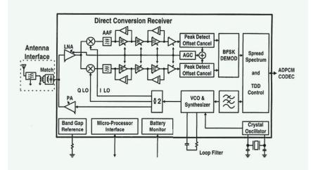
FIGURE 25: A CMOS direct-conversion transceiver reported in 1999 [63]. Demod.: demodulator.
