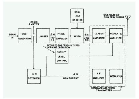
FIGURE 2: Kahn's polar modulation system [5]. AF: audio frequency; KC: kilocycles per second (kHz); Osc.: oscillator; XTAL: crystal.
