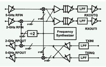
FIGURE 27: A 2.4-GHz/5-GHz direct-conversion transceiver reported in 2004 [78].
