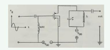
FIGURE 6: A CMOS PA from 1966 [10]. RFC: radio-frequency choke.
