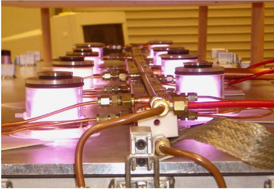
Fig. 55. An 8-tube PM helicon array powered from a rectangular 50\Omega transmission line.
