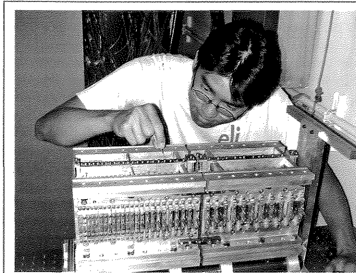
A masterpiece of engineering: The Neptune Lab's unique double-tapered undulator is made of five thousand pieces and was built for an inverse-free electron laser experiment carried out in collaboration with the UCLA Physics Department. Graduate student Jay Sung tunes the undulator.
