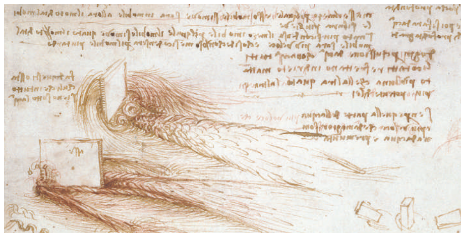
Figure 1 | Turbulent history. A rigid obstacle in flowing water creates wake turbulence, a fact noted and sketched by Leonardo da Vinci in 1509. The passage of a moving body through a static medium has the same effect, and the turbulence can be used to accelerate a following body. What is true for a boat in water also applies to electrons passing through a gas, a fact exploited by Blumenfeld et al. 1 in their high-energy plasma wakefield accelerator.
