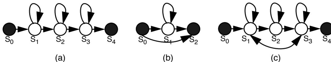
Figure 3.2: HMM models used for acoustic modeling for the Aurora-4 task: (a) typical triphone, (b) short pause, and (c) silence. The shaded states denote the start and stop states for each model. *Figure from [2]*
