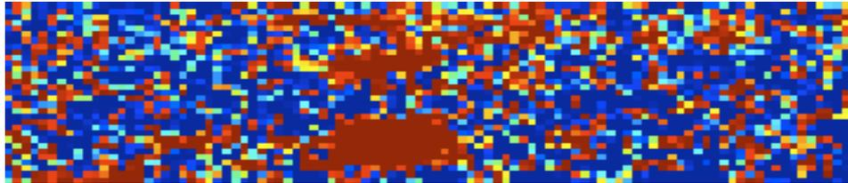
(c) Soft-mask  $M_{i,m}^{(1)}$  after mapping of the SNR to  $[0,1]$  using  $\alpha = 0.2$  and  $\beta = 4dB$
