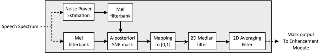
Figure 2.1: Flowchart of the proposed mask estimation technique
