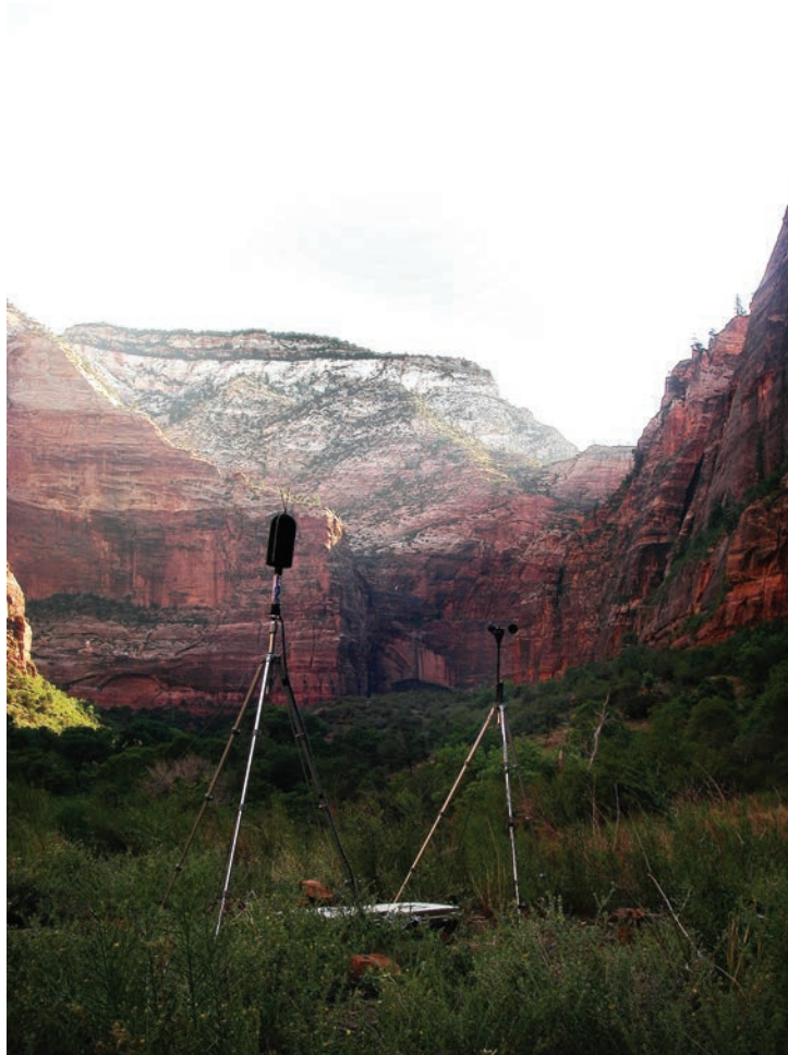
Fig. 1. A National Park Service (NPS) acoustical monitoring system deployed in Zion National Park. Through many generations of NPS systems, wind speed logging has been a consistent component, to identify times when pseudonoise generated by airflow around the wind screen would inflate the spectrum measurements.
