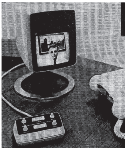
FIGURE 7: The PICTUREPHONE, a video communication device developed at Bell Labs (from [8]).
