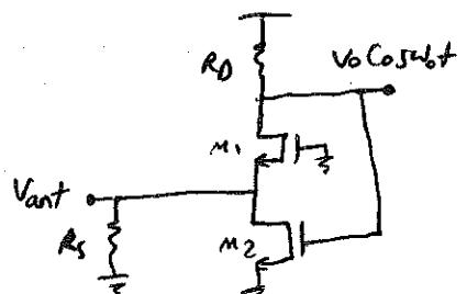
2. A single MOSFET can serve as a "poor man's" mixer. Suppose the device is in saturation and the output of interest is  $I_{out}$ . Neglect channel-length modulation and body effect. Assume the device is characterized by  $I_D = K(V_{RF} - V_{LO})^2$ , where  $V_{LO} = B \cos \omega_{LO} t$ . The LO amplitude is not large enough to cause complete switching.
