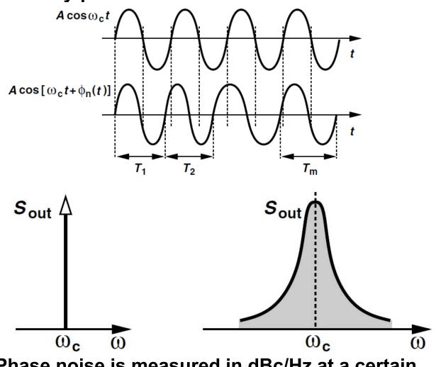
Phase noise is measured in dBc/Hz at a certain frequency offset.
