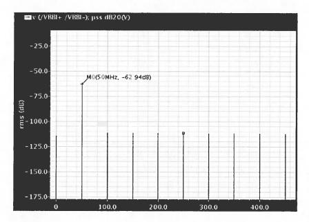
d)The first mechanism of translating 8.7 GHz to baseband is mixing with the third-order harmonic of the LO in first mixer and then mixing with fundamental tone of LO in the second mixer:
