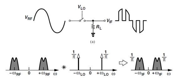
Conversion Gain: How about single-balanced and double-balanced?
