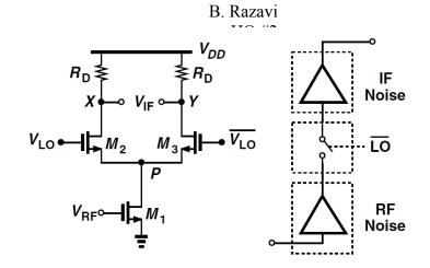
$$\overline{V_{n,X}^2} = \frac{1}{2} \left( \overline{I_{n,M1}^2} \right) R_D^2 + 4kTR_D$$
