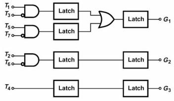
Gray encoding improves the response to bubbles because its accuracy degrades gracefully as the number of sparkles increases:
