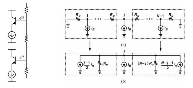
In addition, capacitive paths between the two inputs of each comparator feed part of the analog input to the ladder. This causes <u>ac bowing.</u>
