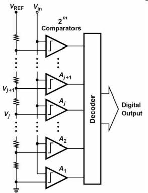
If the comparators are designed as described before, they perform "sampling" in addition to quantization. This is because, at the moment of strobe, each comparator sores with <u>polarity</u> of its input difference.
