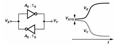
If input is uniformly distributed between  $-V_{XY1}$  and  $+V_{XY1}$ , then the probability that output does not reach  $V_{XY1}$  within T<sub>c</sub> seconds is:
