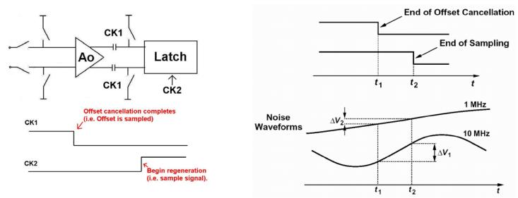
If amplitude of noise components after t1 is correlated (e.g., similar) with that before t1, the noise is also suppressed.
