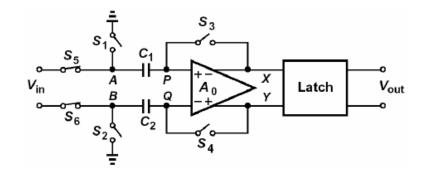
$$V_{os,tot} = \frac{V_{osA}}{1 + A_o} + \frac{\Delta q}{C} + \frac{V_{osL}}{A_o}$$
