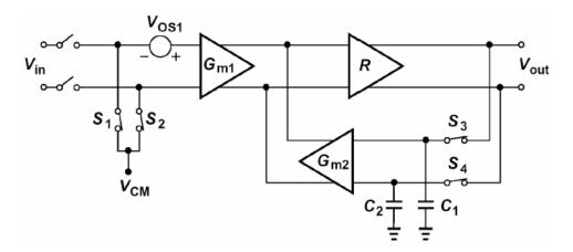
First, assume inputs of  $G_{m1}$  and  $G_{m2}$  are grounded.
