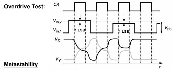
Positive feedback provides infinite gain if given infinite time.
