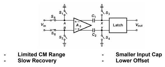
Note: Gain of preamp cannot be very high here because  $V_{\text{OSA}}.A_{\text{o}}$  may saturate the output.
