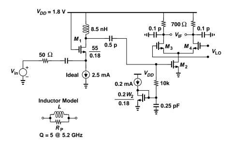
(a) Determine the width of  $M_2$  to obtain resonance at 5.2 GHz.
