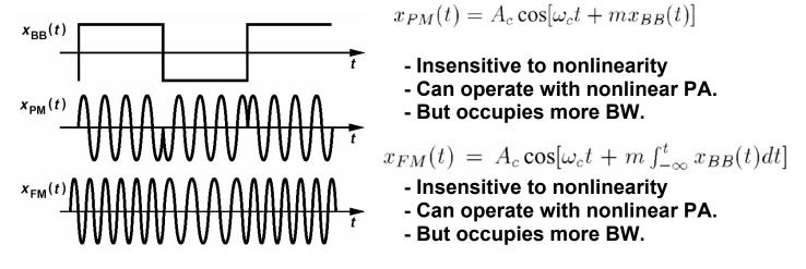
How to build a frequency modulator?
