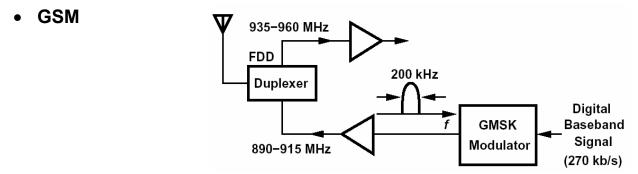
Now we have GPRS and EDGE. EDGE uses variable-envelope modulation and requires a linear PA.
