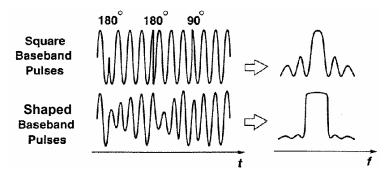
Thus, shaped QPSK has a <u>variable</u> amplitude (envelope) and hence requires a linear PA. GSMK, on the other hand, has a <u>constant</u> envelope and can operate with nonlinear PAs.
