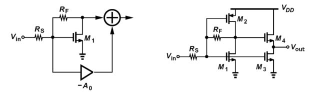
Exercise: Find the NF of the circuit on the left including the inputreferred noise voltage of the additional amplifier.
