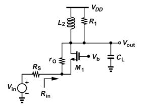
$$\begin{split} \frac{V_{out}}{V_{in}} &= \frac{(g_m + g_{mb})r_O + 1}{r_O + (g_m + g_{mb})r_OR_S + R_S + R_1}R_1 \\ \frac{V_{out}}{V_{in}} &= \frac{(g_m + g_{mb})r_O + 1}{2(1 + r_O/R_1)} \end{split}$$
