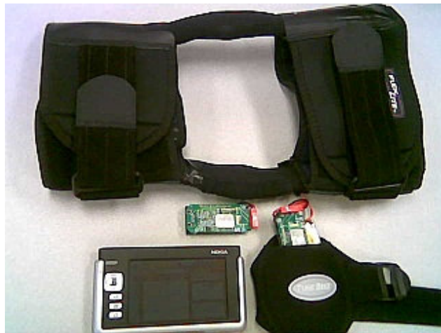
Figure 6: The prototype hardware system includes one base station and two sensor nodes. A knee brace is used for emulating limping context.
