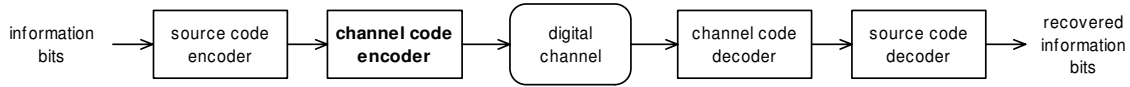
Figure 1. A typical digital communication system. LDPC is considered for the channel encoder/decoder in this paper.
