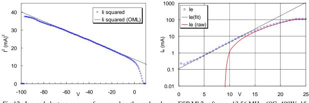
Fig 12. Ion and electron curves of a case when the probe glows. ESP Mk2 software, 13.56 MHz, 60G, 400W, 15 mTorr,  $n = 1.65 \times 10^{12}$  cm<sup>-3</sup>,  $KT_e = 2.72$  eV.
