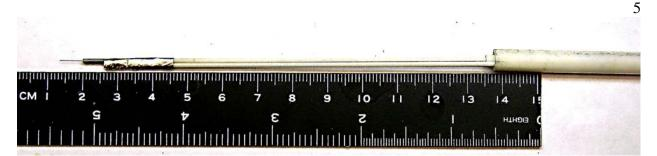
Fig. 4. Photograph of the vertical probe with compensation electrode.
