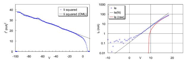
Fig. 13. Ion and electron curves of the plasma of Fig. 12, but taken with ESPion software. The derived *n* is  $1.57 \times 10^{12}$  cm<sup>-3</sup>, and  $KT_e = 2.6$  eV.
