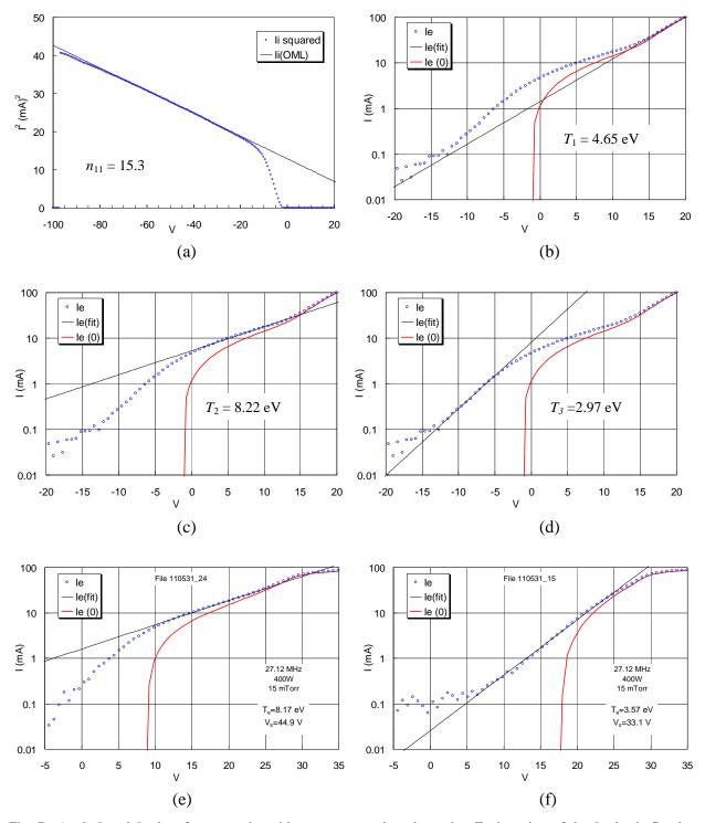
Fig. 7. (a–d)  $I_i$  and  $I_e$  plots from a probe with no compensation electrode. Each region of the  $I_e$  plot is fitted to straight lines to give three different apparent values of  $T_e$ . The discharge was at high field: 280G. (e–f) Example of (d) high  $T_e$  from a poorly compensated and (f) correct  $T_e$  from a well compensated probe in the same plasma.
