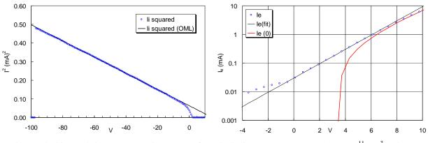
Fig. 9. Ideal ion and electron curves downstream from the helicon source. Here  $n = 0.8 \times 10^{11}$  cm<sup>-3</sup> and  $KT_e = 1.6$ eV.
