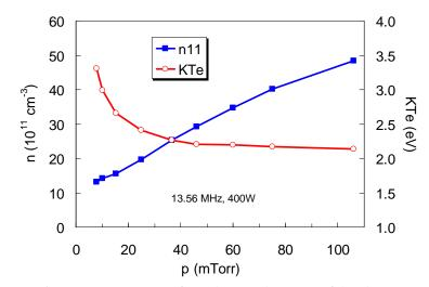
Fig. 17. Pressure scan of n and  $KT_e$  at the center of the plasma.
