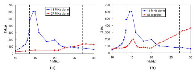
Fig. 5. Impedance measurements of the choke chain (a) before and (b) after connecting the 13-MHz and 27-MHz chokes together. The dashed lines mark the exact RF frequencies.
