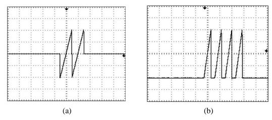
Fig. 6. Voltage sweeps in the Hiden (a) ESP Mk2 and (b) ESPion probe systems. The vertical scale in both is 50V/div, and the horizontal scales are (a) 5sec/div and (b) 25msec/div.
