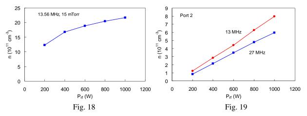
Fig. 18. Power scan with the vertical probe inside the discharge at 13.56 MHz, 65 G, and 15 mTorr. Fig. 19. Power scans at 132 and 27 MHz with a horizontal probe 16.9 cm below the discharge.
