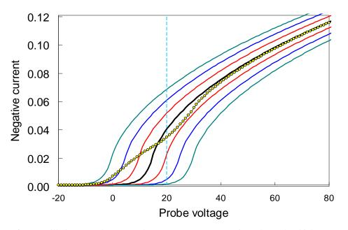
Fig. 1. Effect of RF oscillations on electron probe currents to a Langmuir probe. The thick center curve is the theoretical OML current (amperes) to a probe 0.15 mm in diam and 10 mm long in an argon plasma of density  $10^{11}$  cm<sup>-3</sup>. The shifted I - V curves are for  $V_s - V_p = \pm 5, \pm 10$ , and  $\pm 15V$ . The circles show the DC current averaged over the oscillations.
