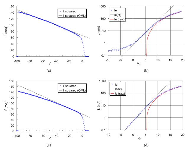
Fig. 10. Example of an I - V curve that shows an electron tail that is not real. The data were taken with ESPion software at the center of the discharge tube at 13.56 MHz, 400W, 65G, and 46 mTorr, and with Scan Average = 50. Analysis yields  $n = 2.92 \times 10^{12}$  cm<sup>-3</sup>, and  $KT_e = 2.21$  eV.
