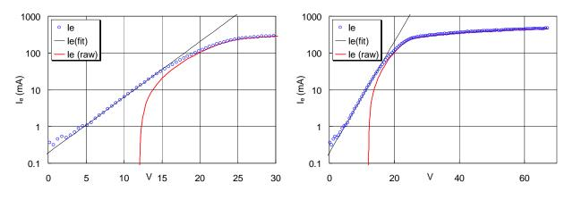
Fig. 15. Electron curves for the  $V_{\text{max}} = +70$ V case shown on two scales. At 2.87eV,  $KT_{\text{e}}$  was normal.
