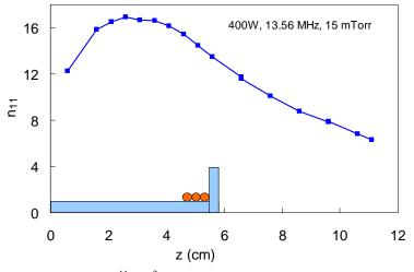
Fig. 16. Axial density profile in units of  $10^{11}$  cm<sup>-3</sup> in a 13.56-MHz helicon discharge at 400W, 15 mTorr of Ar, and a 65G average B-field.
