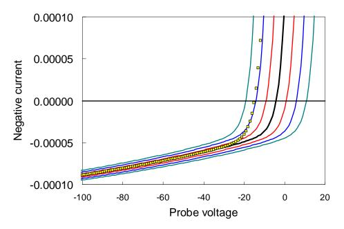
Fig. 2. The ion part of Fig. 1 shown by changing the scales of the plot. The yellow squares (color online) show the time-averaged curve with no RF compensation.
