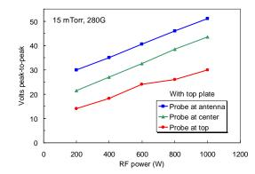
Fig. 8. Peak-to-peak amplitude of RF oscillations in  $V_{\rm f}$  vs.  $P_{\rm rf}$  at three positions in the discharge.
