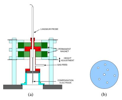
Fig. 3. (a) Schematic of the helicon discharge with a extension chamber to accommodate the vertical probe. The dimensions are to scale. (b) Detail of the top plate with holes.
