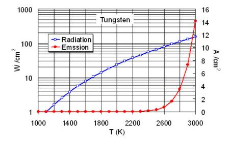
Fig. 11. Optical radiation and electron emission from tungsten vs. absolute temperature.
