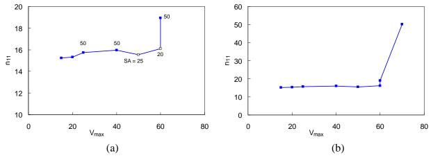
Fig. 14. (a) Ion-derived densities vs. maximum positive  $V_p$  on each scan using ESPion. (b) Same as (a) but extended to Vmax = 70V on a different scale. 400W at 13.56 MHz, 65G, 15 mTorr; probe at center of discharge.
