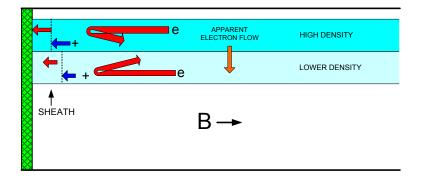
Fig. 2. The short-circuit effect.
