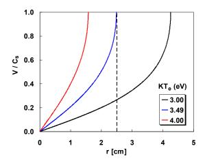
Fig. 5. Profiles of u(r) in a 2.5-cm radius, 10-mTorr argon discharge. Only one value of  $T_e$  gives the right position for the sheath edge.
