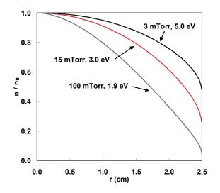
Fig. 7. Density profiles at three pressures, computed with the corresponding  $KT_e$  given in Fig. 5 for a = 2.5 cm.
