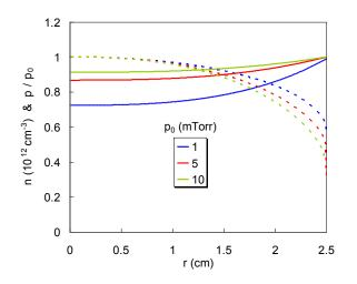
Fig. 8. Neutral pressure profiles (solid lines) for argon discharges in a 5-cm diam tube with initial pressures  $p_0 = 1$ , 5, and 10 mTorr at 400K. The corresponding plasma density profiles peaked at  $10^{12}$  cm<sup>-3</sup> are shown by the dashed curves.
