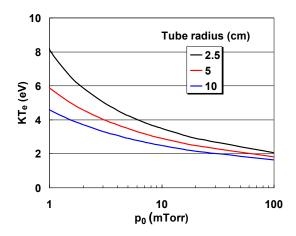
Fig. 6. Relation between  $T_{\rm e}$  and pressure in argon discharges of various radii.
