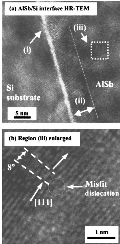
FIG. 2. Cross-sectional HR-TEM image of the AlSb/Si interface, showing the (110) plane. (b) Magnified section of part (a), showing a change in crystallographic orientation and a misfit dislocation that results from it.
