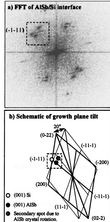
FIG. 3. Fast Fourier transform of a HR-TEM image of AlSb/Si interface. (b) Schematic of (a), showing the presence of an additional AlSb lattice rotated by  $20^\circ$  clockwise to the (100) plane. The  $(-1-11)$  component has been used to illustrate the effect.
