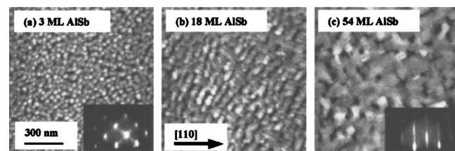
FIG. 1. AFM images showing surface structure after (a) 3 ML, (b) 18 ML, and (c) 54 ML of AlSb deposition on Si. (a) and (c) RHEED images for the corresponding growths.
