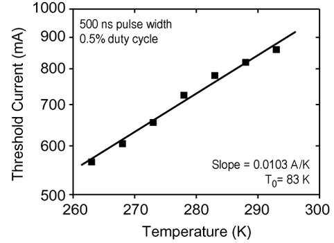
Fig. 3. Threshold current versus stage temperature characteristics of laser. The slope of the curve yields a room-temperature  $T_0$  value of  $83$  K.
