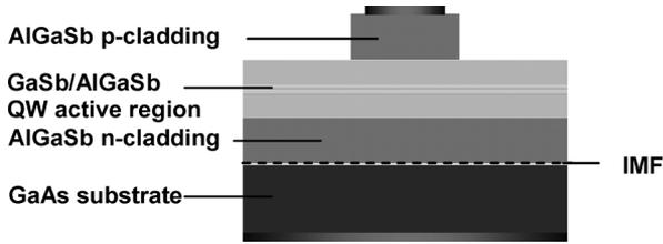
Fig. 1. Device structure for buffer-free GaSb–AlGaSb QW laser grown on a GaAs substrate using an IMF array.
