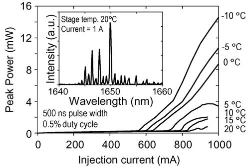
Fig. 2.  $L$ – $I$  characteristics and lasing spectrum for hybrid laser over temperature ( $-10$  °C to  $20$  °C) for a device  $50$   $\mu\text{m}$  in width and  $580$   $\mu\text{m}$  in length.
