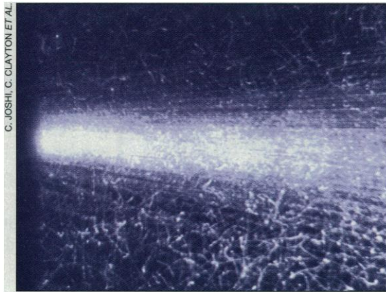
Little big accelerator. Tracks in a cloud chamber indicate paths of electrons accelerated in a plasma wave.
