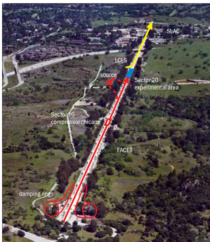
Fig. 1. Aerial view of SLAC showing the location of FACET, which will use the first 2 km of the main linac (red) to deliver high-energy electron and positron beams to a new experimental area (blue). The LCLS X-ray laser (yellow) uses the final kilometre of the SLAC linac. (Image credit: SLAC.)
