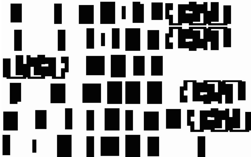
Figure 8: Trim-mask layout snippet where simple large blocks correspond to cells with unidirectional poly and more complex shapes correspond to flip-flops with bidirectional poly-routing.
