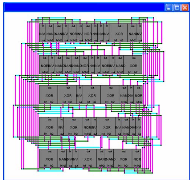
Fig. 8 PRS displaying the layout of a circuit that computes the absolute value of the difference between two 2-bit numbers
