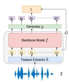
Fig. 1. Proposed self-supervised learning framework. h is a function to extract speech representation Z. O is an operation over Z. f is the backbone model for pretraining. g is a generator that maps the output of the backbone model to have the same dimension as O(Z) and outputs Y. L computes the SSL loss using Y and O(Z).
