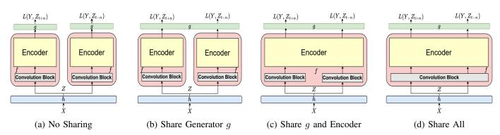
Fig. 2. Various solutions for training a non-causal transformer with Bi-APC. Each color represents one module. Notations and blocks are consistent with those described in Section II.
