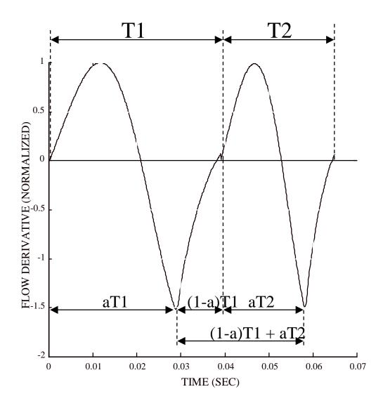
Figure 5.1. Measured synthetic fundamental period combines portions from two separately synthesized pulses; time between minima is measured: the last part of pulse T1, with length (1-a)T1, is combined with the first part of pulse T2, with length aT2. The resulting sum of two random variables is subject to basic rules of error propagation.
