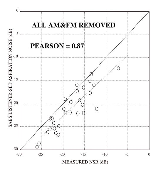
Figure 5.8. Mean of listener-set aspiration noise in SABS experiments versus NSR of voices with all AM and FM removed. Agreement between SABS and measured NSR improves further over Fig. 5.6. Dashed line shows best linear fit.
