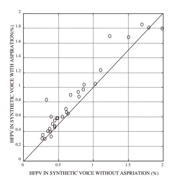
Figure 5.4. Effect of AN on measured HFPV in the synthetic voice. Horizontal axis is programmed HFPV level. Vertical axis is HFPV measured in synthetic voice when the original measured level of AN is added. AN seems to add about 0.2% to the HFPV measurement for the levels found in the voice set.
