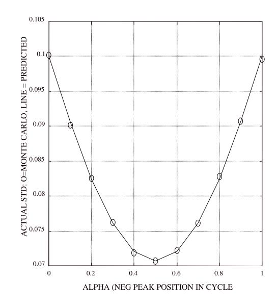
Figure 5.2 . Simulation demonstrating the effect of fundamental peak position on standard deviation of measured fundamental period length. Circles show average simulated result using 100,000 random pulses. Line shows predicted values.
