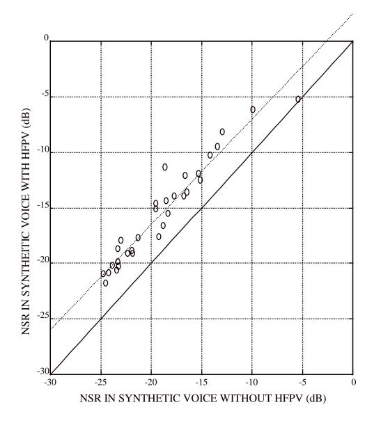
Figure 5.5 Effect of HFPV on measured NSR in the synthetic voice. Horizontal axis is programmed AN level. Vertical axis is measured NSR in the synthetic voice when the original measured level of HFPV is added. HFPV seems to add about a 4 dB increment in NSR for the levels found in the voice set. Dashed line shows best linear fit.
