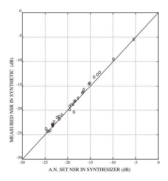
Figure 5.3. Verification of NSR level in synthesized voice. Aspiration noise (AN) levels programmed predict measured levels within about 1 dB.
