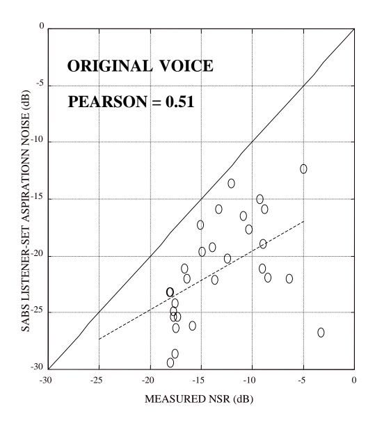
Figure 5.6. Mean of listener-set aspiration noise in SABS experiments versus the measured original NSR. The listeners set AN levels 5 - 10 dB below measured, indicating original NSR includes more than AN effects. Dashed line shows best linear fit.
