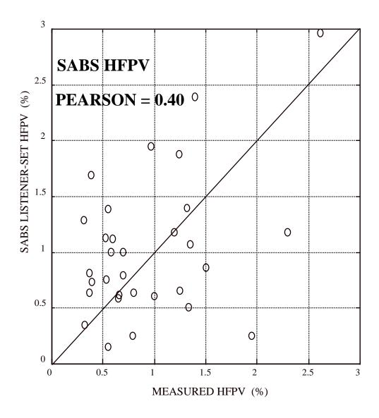
Figure 5.9. SABS comparison of user set HFPV versus measured HFPV. Weak correlation indicates listener difficulty perceiving HFPV at the levels present in the voice set.
