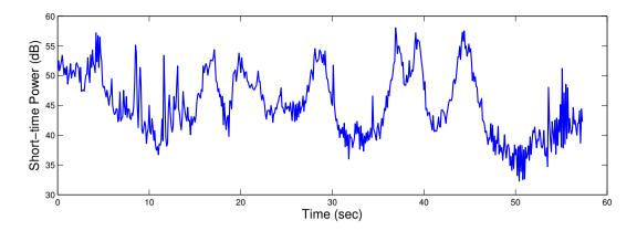
Figure 3.3: The short-time spectral power of pure street noise is highly non-stationary
