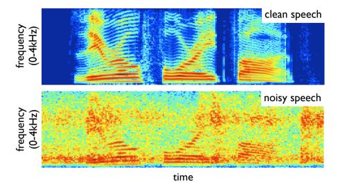
Figure 1.4: The spectrogram of an utterance corrupted by artificially adding subway noise at 0dB SNR (bottom) is highly distorted compared to the spectrogram of the corresponding clean speech utterance (top)
