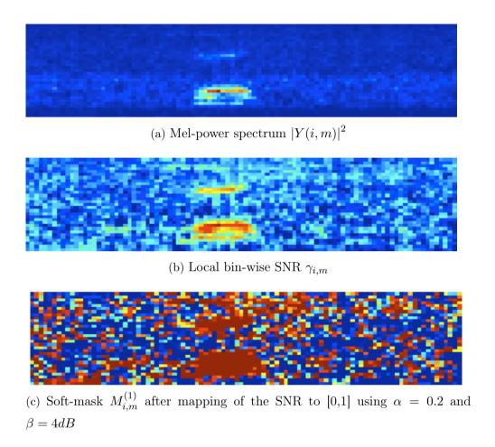
Figure 2.3: Output at the first three steps of the processing of the soft mask for the spoken digit six corrupted by car noise at a global SNR of 5dB. The x-axis corresponds to time and the y-axis to the Mel channel. While the dynamic ranges of these plots differ, blue always corresponds to a value at the lowest-end of the range while red is at the highest-end of the range
