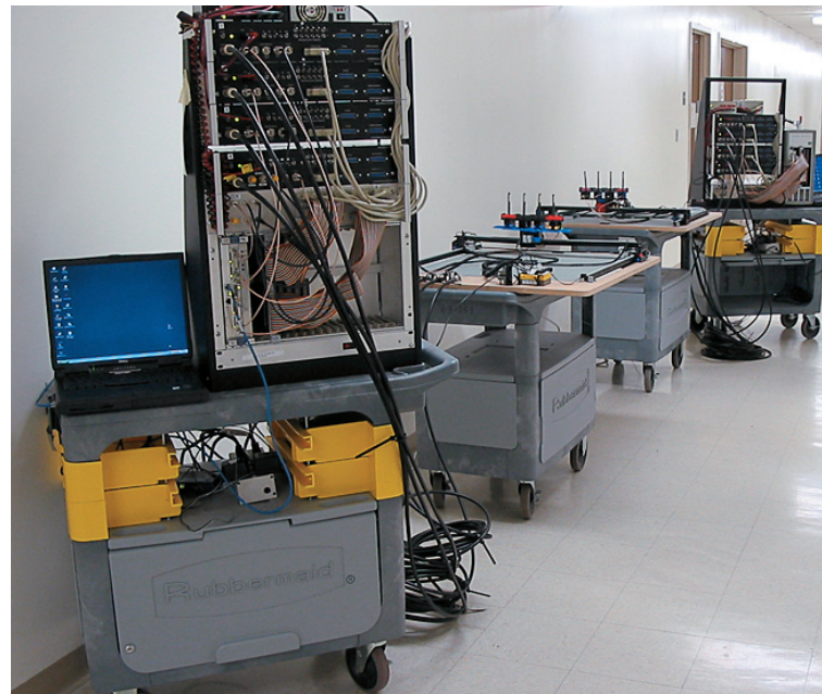
The UnWiReD wideband radio testbed is composed of two multi-antenna radios (far left and right) and two positioning robots (middle) – all of which are remotely controllable over the internet.
