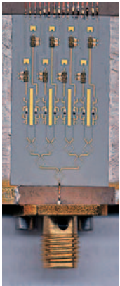
A 60GHz retro-directive array.
