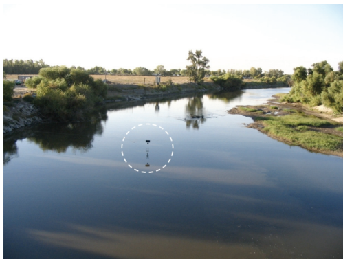
The NIMS robotic sensor system deployed in a 200 foot span across the San Joaquin river near the confluence of the San Joaquin and Merced Rivers (upper left). The NIMS sensor node (indicated by the circle) is seen at the middle of the river as it scans from one river bank to the other. A view from bank to bank is shown at the right.
