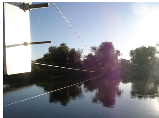
The NIMS robotic sensor system deployed in a 200 foot span across the San Joaquin river near the confluence of the San Joaquin and Merced Rivers (upper left). The NIMS sensor node (indicated by the circle) is seen at the middle of the river as it scans from one river bank to the other. A view from bank to bank is shown at the right.
