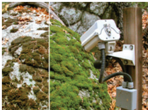
CENS Mosscam used as a physiological sensor (dry season vs wet season).
