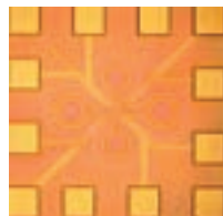
CMOS VCO designed by Prof. M.C. Frank Chang's group at UCLA, fabricated in 90nm process
