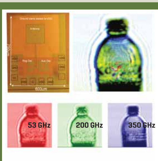
A CMOS 350 GHz color THz imaging receiver developed at UCLA.
