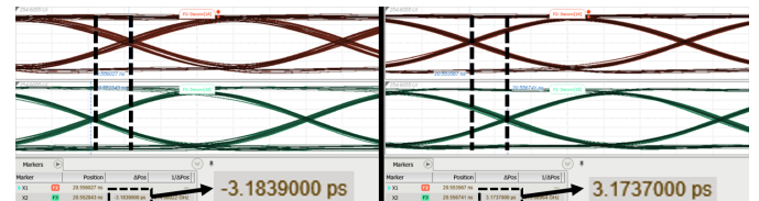
Fig. 6. Single-ended eye diagrams with skew adjustment.
