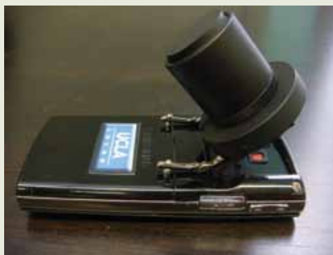
The figure shows a regular cell phone that is converted into a microscopic imager through lensfree holography.
